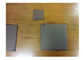
Slotted joints can be very effective depending on where your structure bears weight. Tip: When cutting slots, make sure they're not bigger than the thickness of the material, otherwise your joint will be very loose and unstable.
