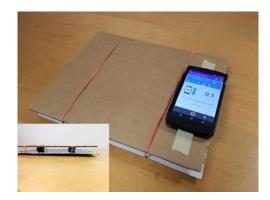
Make sure the Science Journal app is measuring acceleration in the appropriate direction and give it a test. You should be able to get at least 6 m/s2 (meters per second squared) worth of vibration from your simulator.
